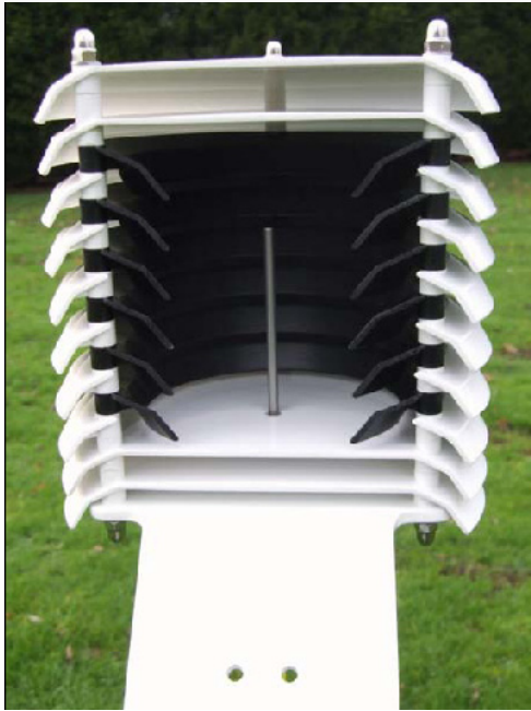
A cross-sectional cutaway showing the external and internal louvres of the larger capacity MET20 shield
