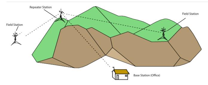
Our RF networks require line-of-sight transmission. The mountain in this drawing obstructs line-of-sight with the base station. Use of the repeater station allows the base station to receive data from the field stations.
