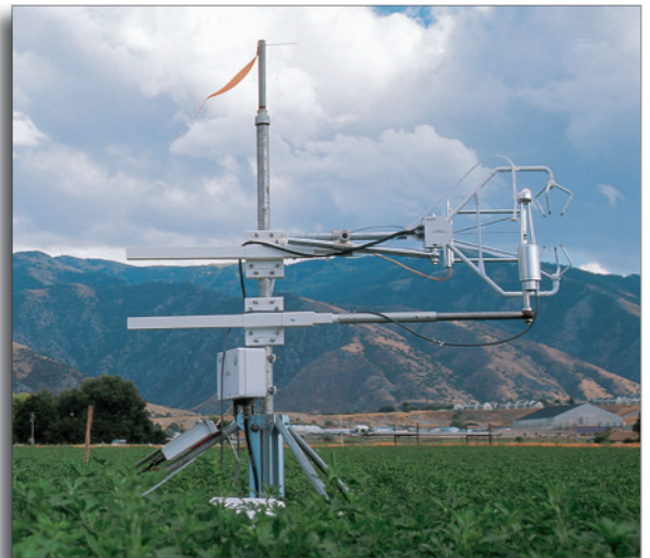
An integrated eddy covariance station monitors CO 2 and water vapor fluxes over an alfalfa field.
