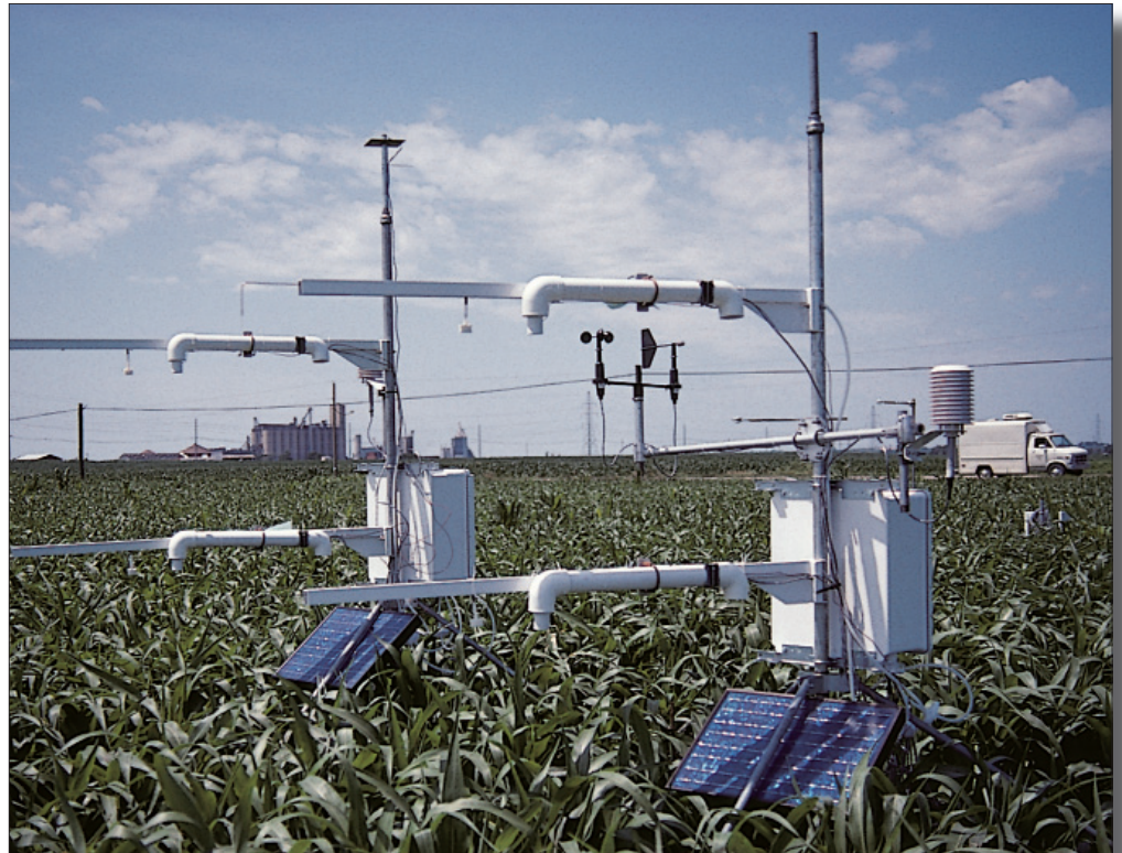
Two Bowen ratio systems calculate evapotranspiration and CO 2 fluxes over a sorghum field near Lincoln, Nebraska.
