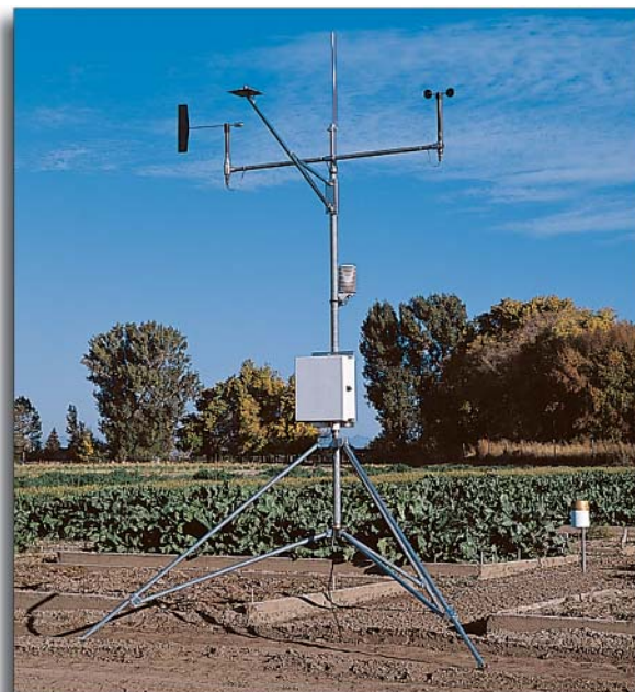
In addition to meteorological parameters, the station also monitors soil water content via probes located throughout the agricultural plot.
