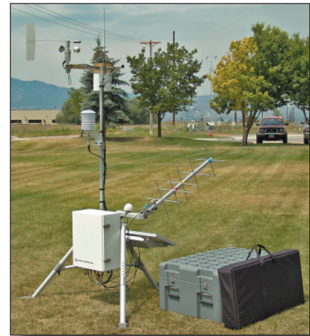
The components of a RAWS-F station fit inside of two optional carrying cases for easily transporting the station to the site.
