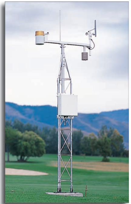
ALERT stations, hybrid ALERT stations, customized water quality/stage stations, and weather stations can all supply data to a LoggerNet-based system.
