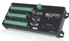
The CR1000 provides adequate inputs for most hybrid flood monitoring stations.
