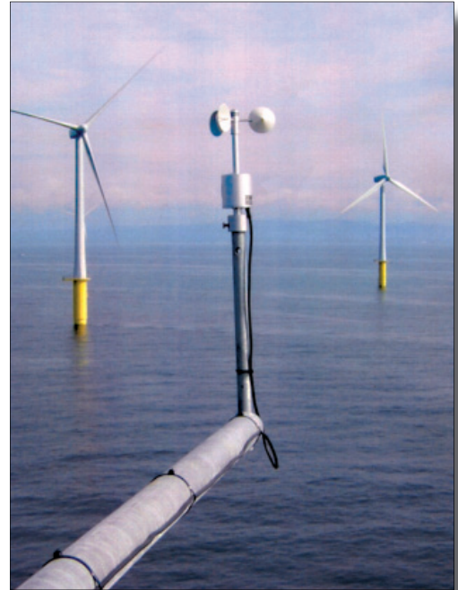
View from one of the anemometers on the meteorological tower to the monopiles and turbines of a wind farm (photo courtesy npower renewables).
