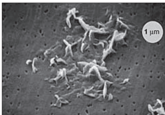
Figure 1. This Scanning Electron Microscopy (SEM) image shows that formazin particles have many different shapes.
