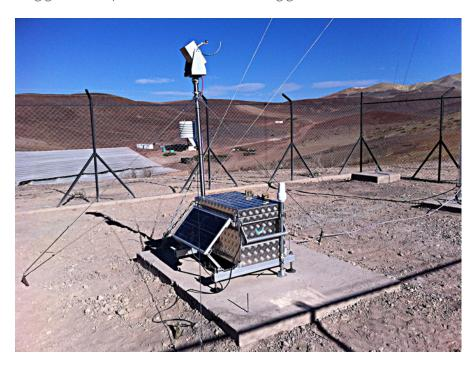
Solar energy resource assessment projects are critical to the successful siting of solar thermal power plants. Before a plant is developed, the environment of the plant's intended location must be studied in detail to ensure that the site will continue to deliver a consistent and reliable source of solar power. If it is determined that a site cannot harness a continuous and sufficient solar-energy supply, another site must be selected and researched.
