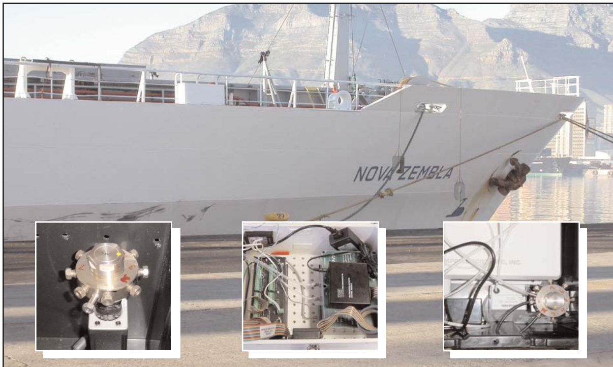
The instrumented citrus transport ship sits at the dock awaiting departure. Inset photos: the rotary valve, datalogger, CO 2 analyzer, and tubing.
