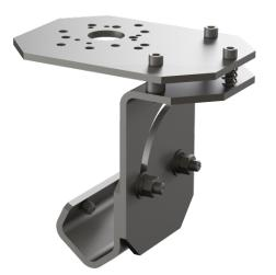
Solar radiation sensor mounts attach to tripods or towers, while providing a sturdy, level platform for pyranometers, quantum sensors, and radiometers. Some solar radiation sensors may also require a leveling base that incorporates a bubble level and three adjusting screws to level the sensor.
