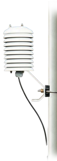
FIGURE 7-1. Installing a 107 and RAD10 Radiation Shield on a vertical pole
