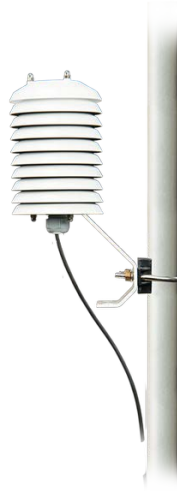
FIGURE 7-1. Installing a 109 and RAD10 Radiation Shield on a vertical pole
