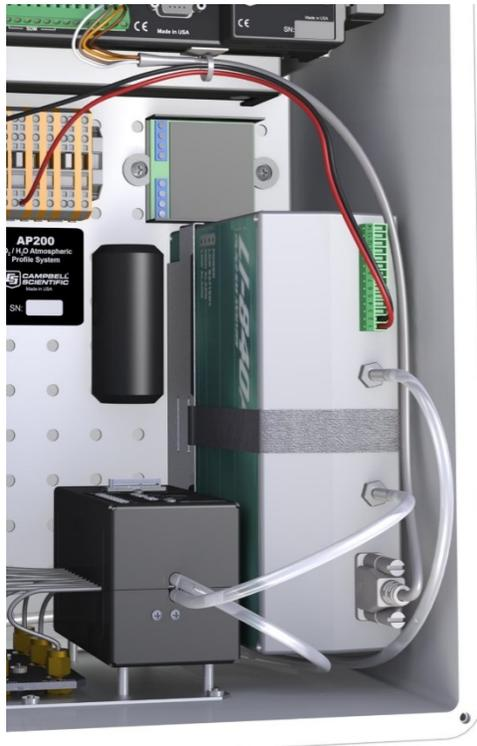
FIGURE 7-4. Installed IRGA in system enclosure
