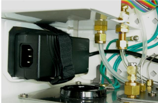
FIGURE G-1. Installation location of power adapter
