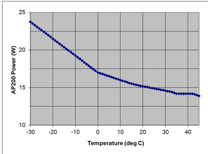
FIGURE 4-23. Average power consumption relative to temperature
