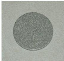
FIGURE 4-13. Disk filter of early AP200 intake assembly
