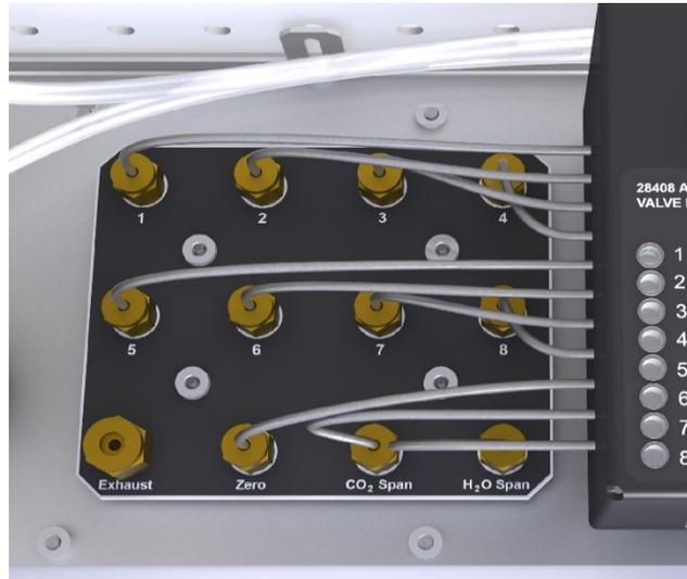
FIGURE 5-6. Labelled inlet connections inside enclosure
