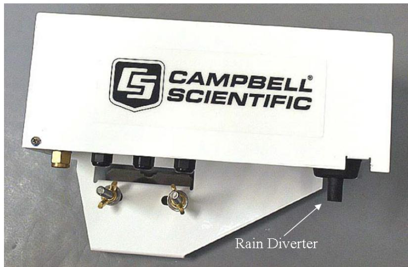
FIGURE 4-2. Side view of AP200 intake assembly
