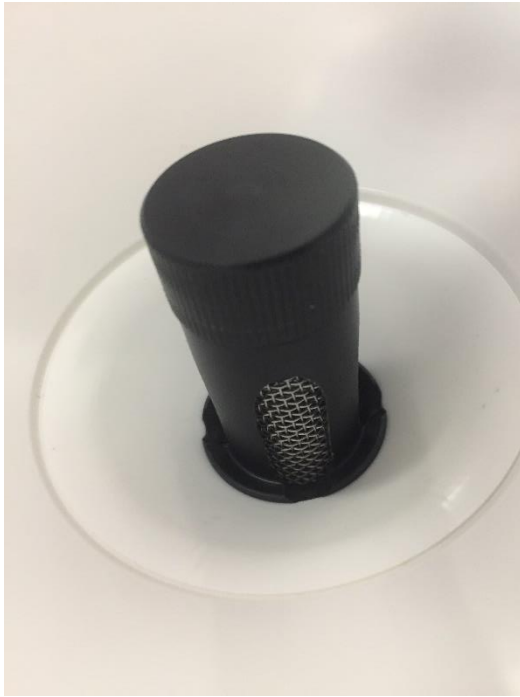
Figure 3 - Filter and filter cap (left) / Nozzle delivering water into tipping bucket (right)
