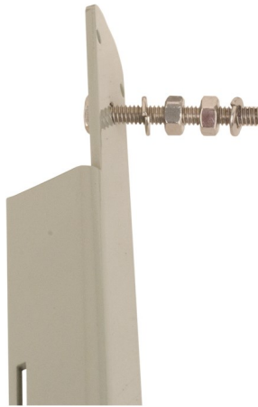
Figure 7-2. Nuts and lock washers on mounting bolt
