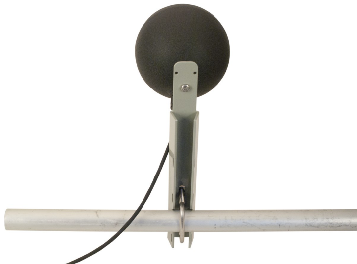
Figure 7-5. BlackGlobe mounted to a crossarm (back view)
