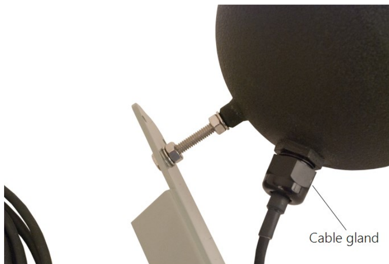
Figure 7-3. BlackGlobe fitting and cable alignment
