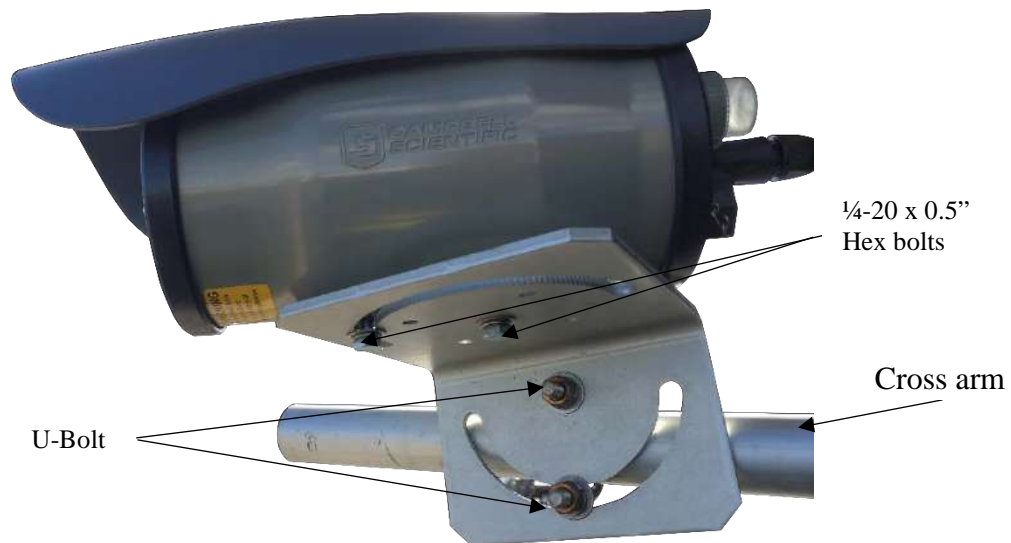
Figure 21-3 CCFC Mounted to Cross arm
