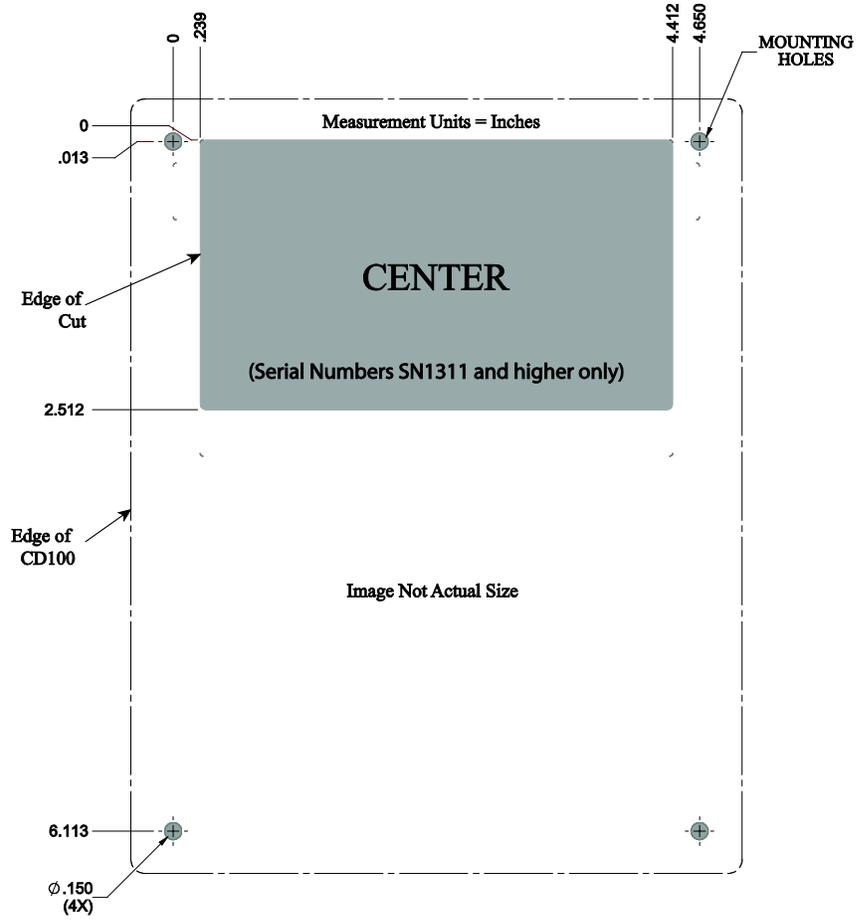
FIGURE 6-2. Template measurements for serial numbers 1311 and higher
