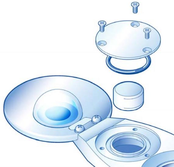
FIGURE 8-3. Replacing Drying Cartridge
