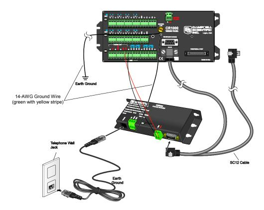
FIGURE 6-3. COM320 Grounding and Alternate 12Vdc Power
