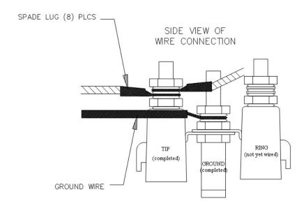
FIGURE 6-5. Side View of Surge Suppressor Wiring
