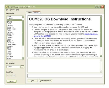
FIGURE B-1. Send OS Screen in Device Configuration Utility
