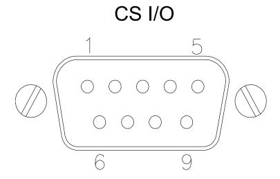
FIGURE C-1. COM320's Male 9 Pin Connector
