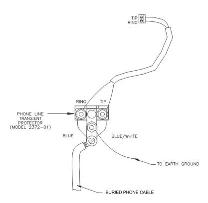
FIGURE 6-4. Top View of Surge Suppressor Wiring
