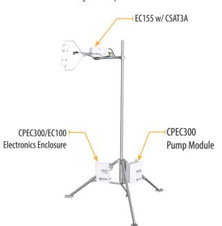
4. Connect the EC155 and CSAT3A to the electronics.
