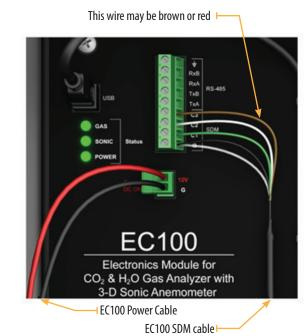
Draw the EC100 power cable and EC100 SDM cable through the feedthrough at the bottom of the CPEC306 enclosure and connect them to the DINrail.
