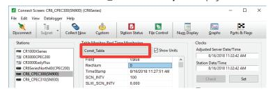
Confirm all the sensors used at the site are set to -1. To change a value in this table, right-click on the current value and select View/Modify from the pop-up menu. Press Apply once the new value has been entered.
