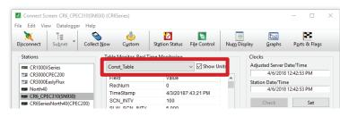
3. Set the variables listed below to enable auto zero and span. -1 indicates true and 0 indicates false. ZRO S days be ZRO S the aut
