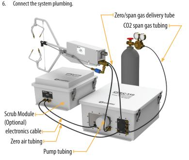
Note: A zero gas cylinder can be used in place of the scrub module to provide zero gas for zeroing the analyzer.
