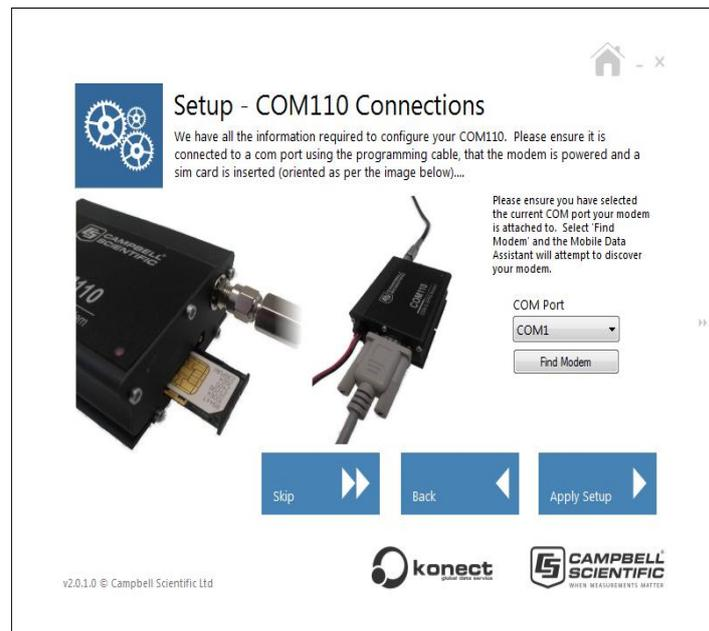
If you are unsure which serial port on your PC the modem is connected to, you can click on the Find Modem button. It is quicker though, if you know the serial port, to set the com port. Then click on Apply Setup. The program will then send the required settings to the modem to configure it. At the end of this process, which takes a minute or so, the program should report it has setup the modem correctly. Then click on “Done”.
