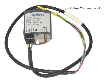
FIGURE 7-3. CS100 and cable with warning label
