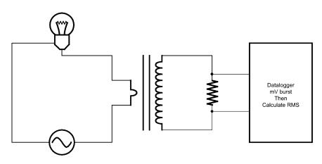
FIGURE C-2. Schematic of generator with current transformer
