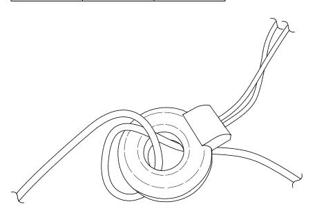
FIGURE C-9. CS11 with the AC wire making two passes through the CS11
