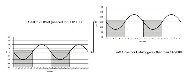
FIGURE C-7. Adding 1250 mV creates positive output
