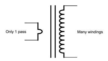
FIGURE C-6. Windings schematic
