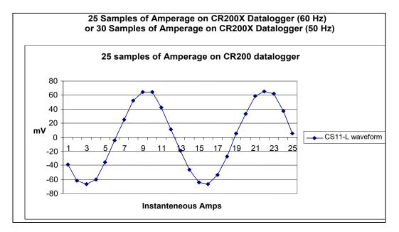
FIGURE 7-3. Graph of a CS11 waveform
