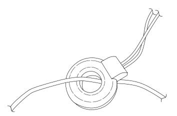
FIGURE 7-1. AC load wire installed in CS11
