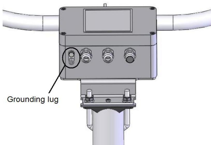
The CS120 must be properly grounded by taking a ground wire with a minimum cross sectional area of 6 mm<sup>2</sup> and maximum length of 5 m from the brass grounding lug in the lower face of the electronics enclosure to an adequate grounding point. The pole and foundations of a pole mounted installation will provide some basic lightning protection and protection against radio frequency interference and should also be correctly grounded.
