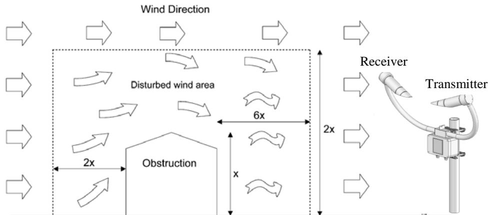
In order to reduce the service frequency with the unit, the CS120 should be placed away from sources of contamination, in the case of roadside monitoring; larger mounting poles can be used. More regular maintenance will be required when the instrument is placed in areas where contamination is unavoidable or where measurements may be safety critical.
