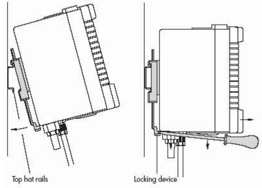
FIGURE 4-1. Securing the CS470 to a Hat Rail
