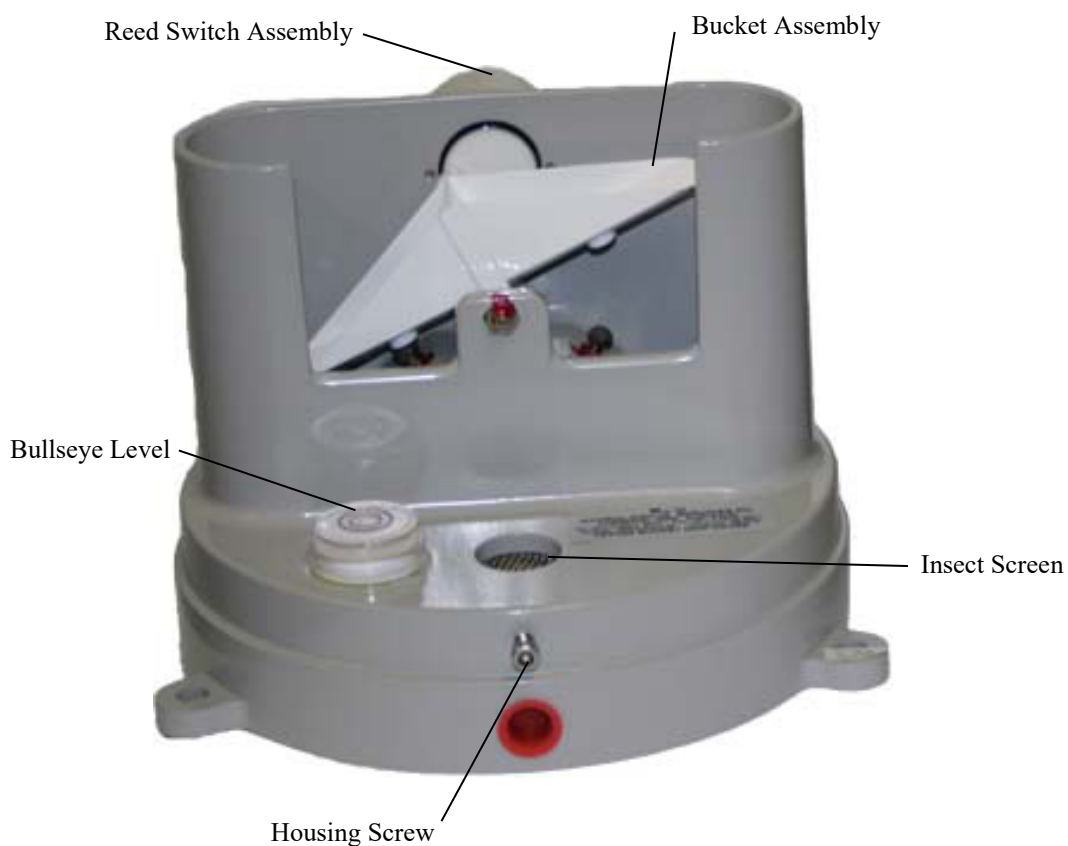
FIGURE 9-1. Components of CS700 Base
