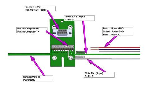
FIGURE 4-1. CS725 connection to DB9F-TERM
