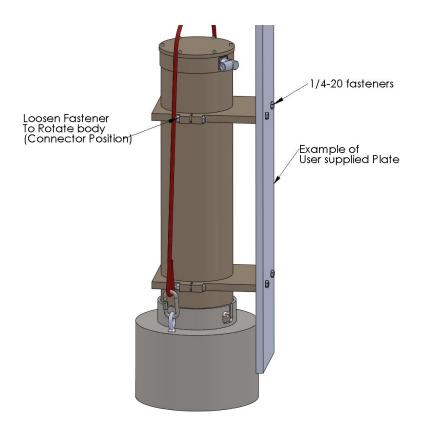
FIGURE 9-2. Example of wall/plate mounting
