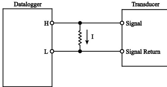
Ohm's law describes how a voltage (V) is generated by the signal current (I) through a completion resistor (R):
