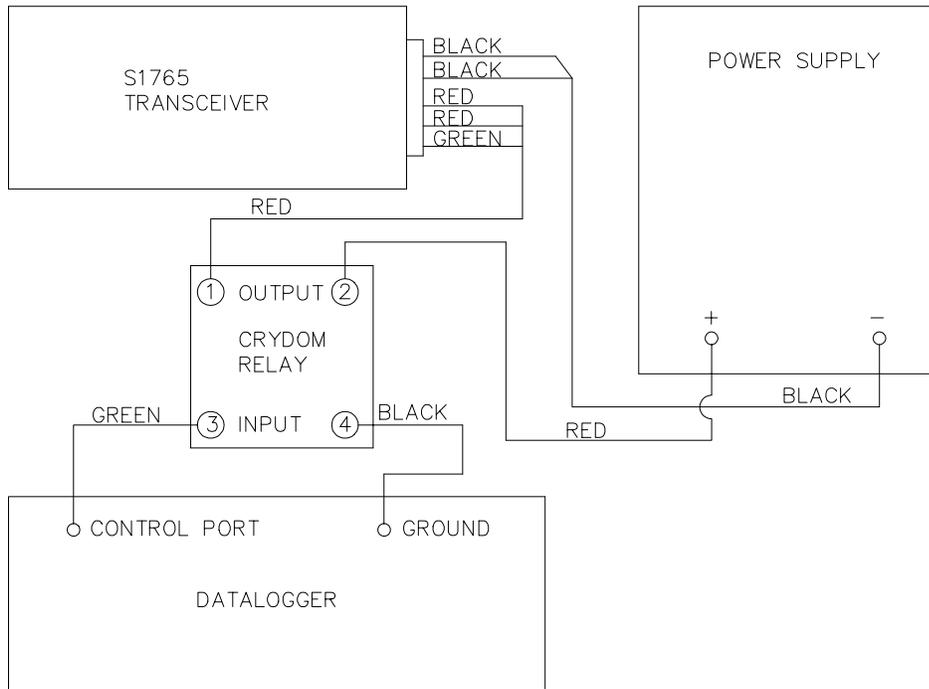
FIGURE 5-1. DC1765 Wiring
