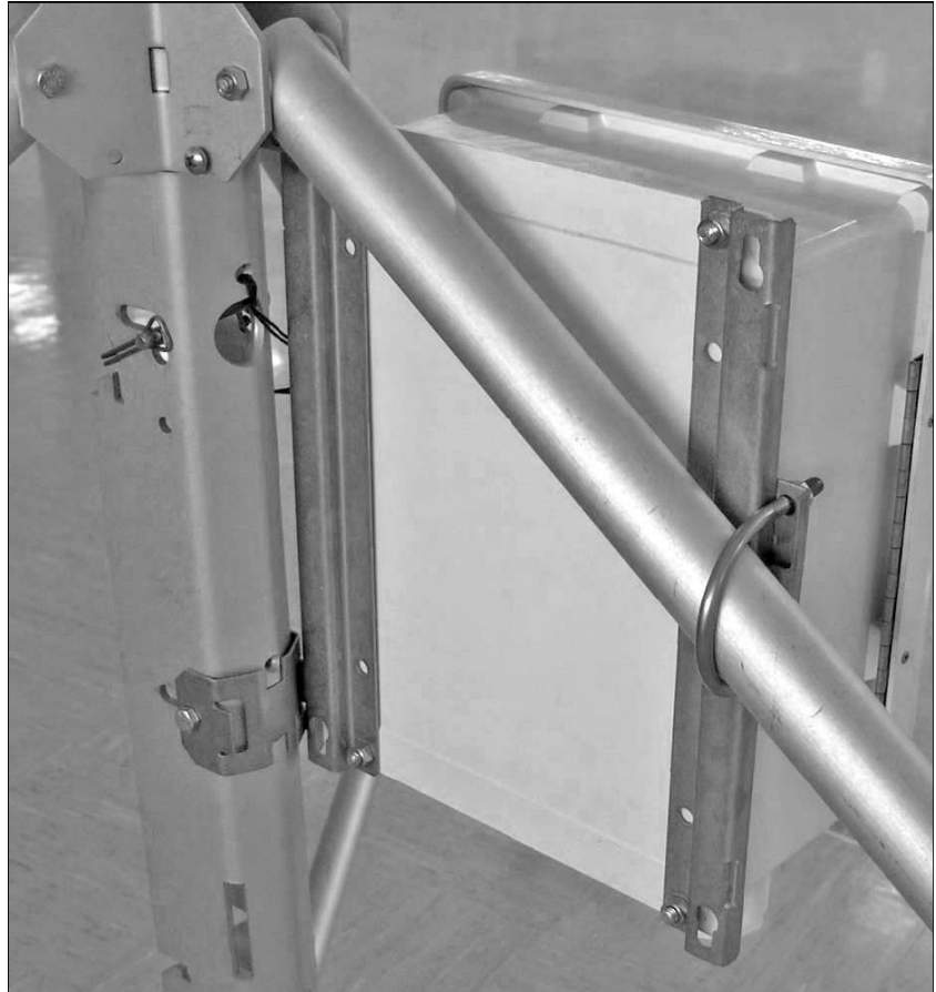
Figure 7-10. An enclosure attached to the leg base of a CM110 tripod.
