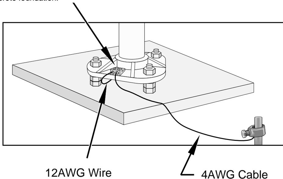
**FIGURE 2.2-1. Raising and Grounding the ET Tower**
