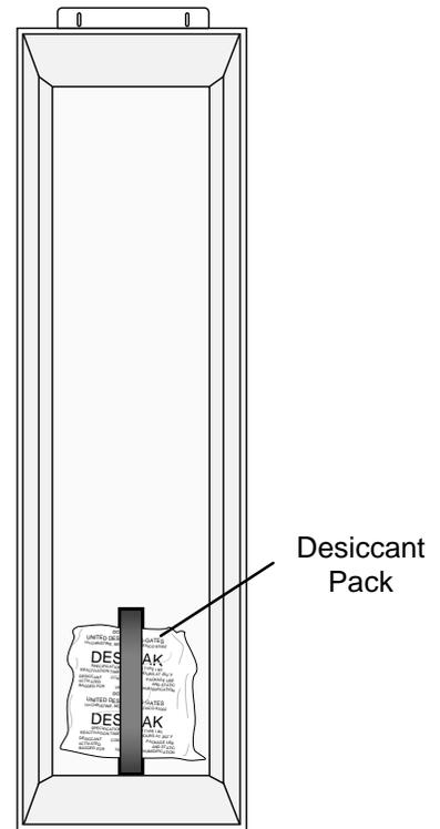
FIGURE 3.4-1. Desiccant Installation
