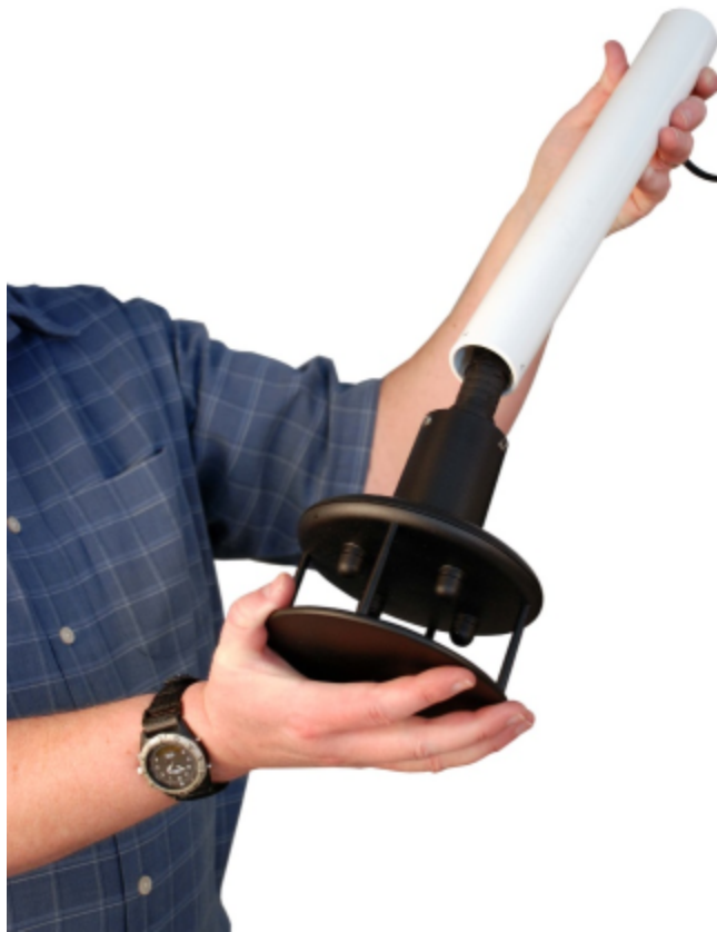
FIGURE 6-17. WindSonic connected to cable
