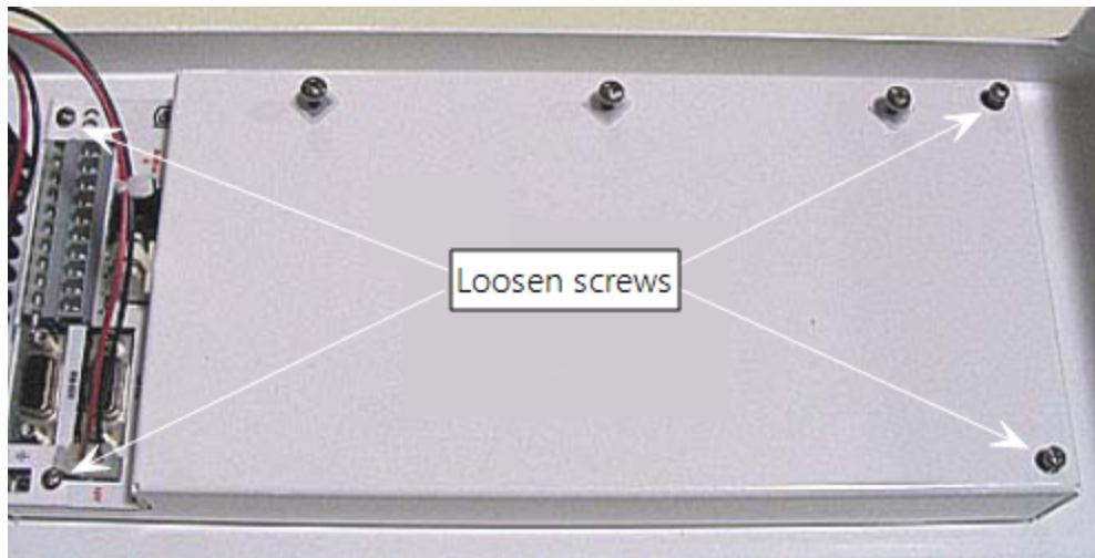
FIGURE 6-13. Screws that secure the electronics cover
