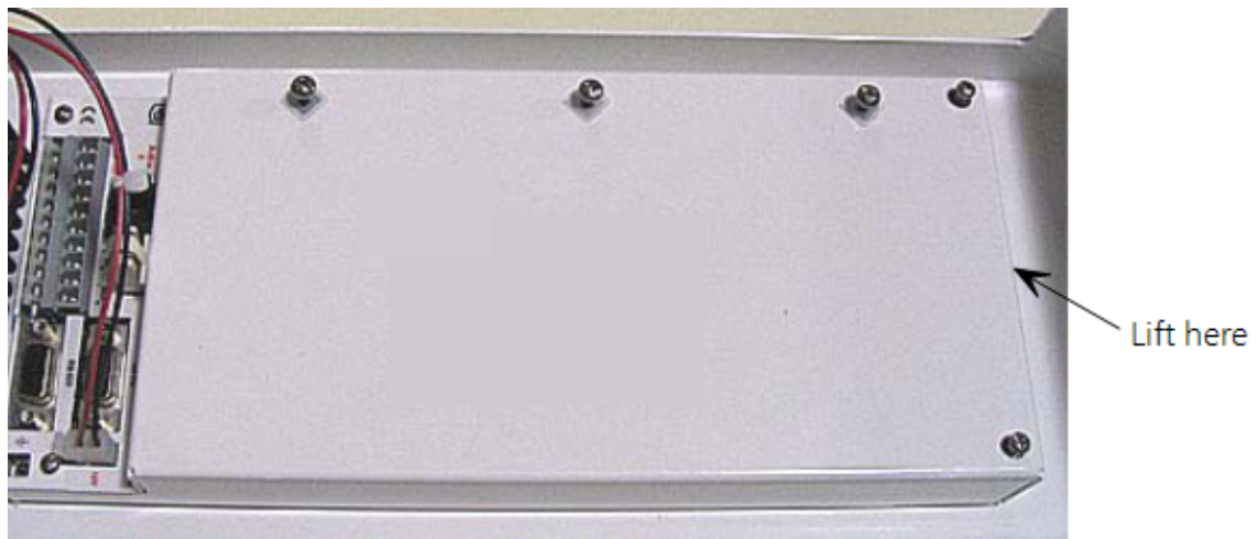
FIGURE 6-14. Removal of the electronics cover
