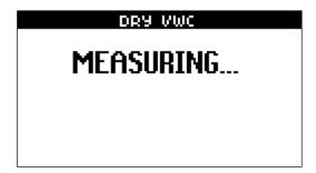
The screen will show MEASURING... while the measurement is taken. After 3 to 4 seconds, the soil profile page will be shown with the reference value changed. Repeat this process for the remaining wet or dry set point.
