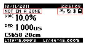
When the current position is not within an existing zone, **NOT IN A ZONE** is displayed. When the HydroSense II is moved within the boundaries of an existing zone (such as ZONE 00001 in the following figure), the zone name will be displayed.
