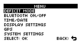
To enter the main menu, press MENU from the *main screen (p. 15)*. Using the buttons, select the desired menu item and press OK. To exit the menu, press STORE.
