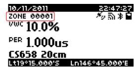
Zones can be created when data are stored. When the *Store* (p. 14) button is pressed, and the HydroSense II determines that the current location is not in an existing zone, **CREATE A NEW ZONE?** is displayed.
