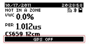
If the GPS is turned off using the *configuration menu (p. A-1)*, GPS OFF is displayed at the bottom.
