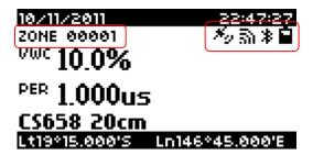
This change occurs automatically when the HydroSense II detects that it is within the boundaries of a zone. For more information on zones, please see Section 9.2, *Geotagging and Zones (p. 20)*.
