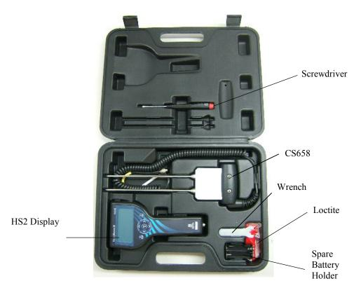
FIGURE 4-1. HS2 Parts in Hard Carrying Case
