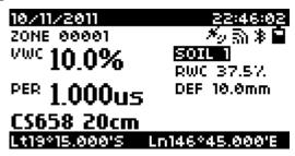
When Deficit Mode is enabled (Section 7.3.4, *Deficit Display (p. 17)*), soil profiles are accessed from the *main screen (p. 15)* of the HydroSense II. To select the current soil profile ("SOIL 1" in the preceding figure), press the button. The soil profile number will be highlighted. To open the soil profile
