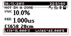
The top bar of the screen displays the current date and time information. This time is synchronized with the GPS when available. The bottom bar shows the current GPS coordinates. Both values are updated automatically.
