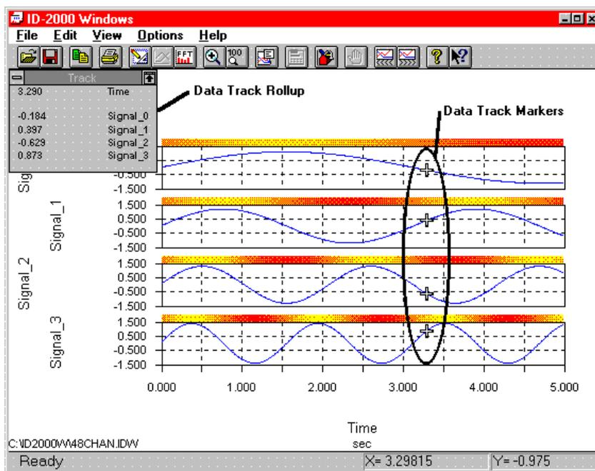
**FIGURE 3-13. Data Track Rollup and Data Track Markers**
