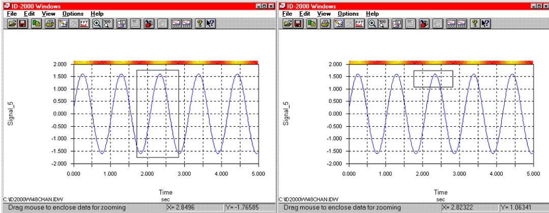
FIGURE 3-4. Zooming Strip Charts using Time and Autoscaling
