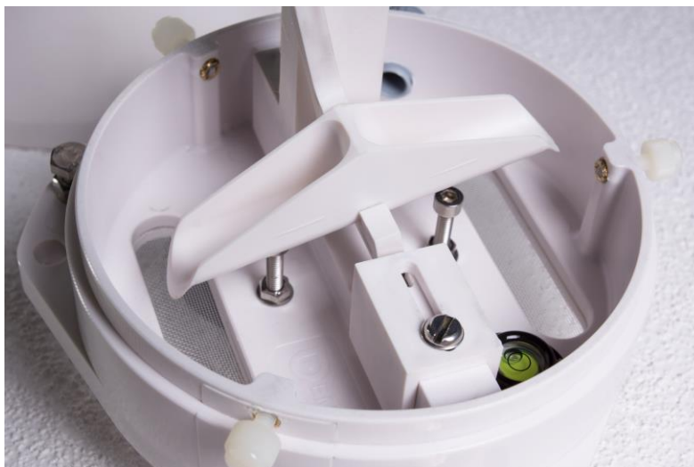
Figure 2. Internal view of the Kalyx showing the tipping bucket mechanism and level indicator.
