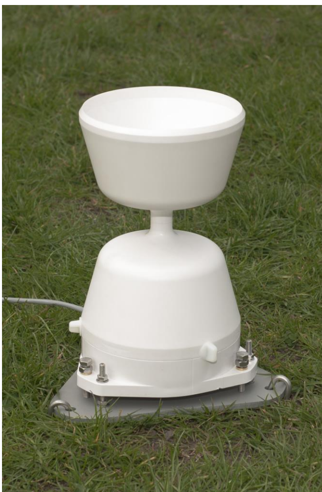
Figure 3. The Kalyx gauge fitted on the ground mounted baseplate that is held down with pegs/stakes.
