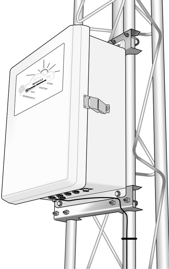
**FIGURE 3.1-2. MetData1 Enclosure on UT10 or UT30 Tower**
