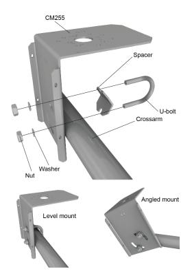
5. For the CM256 bracket, use the two set screws to secure the bracket to the crossarm or pole as shown in the following figure. For pyranometers mounted horizontally, ensure the mounting bracket is horizontal in two dimensions. For pyranometers mounted at an angle, set the mounting bracket angle to the desired angle prior to tightening the mounting hardware.
