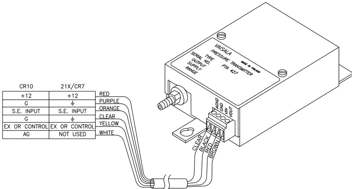
WHITE is not used on the 21X or the CR7 installation; it should be taped or cut to protect from shorting.
