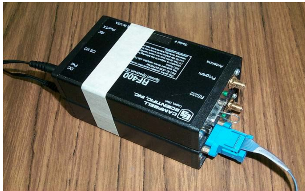
FIGURE K-1. Loop-back Test without Antennas
