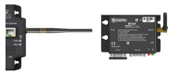
2. For data loggers with an external radio, connect the radio and data logger **CS I/O** ports using an SC12 cable.
