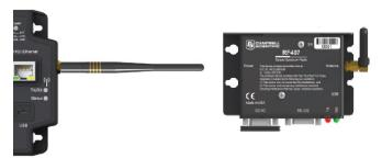
2. For data loggers with an external radio, connect the radio and data logger **CS I/O** ports using an SC12 cable.
