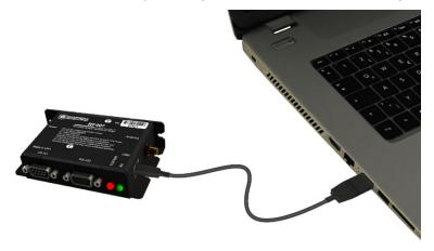
4. Using *Device Configuration Utility*, select the Communication Port used for your radio and connect to the RF407-series radio.
