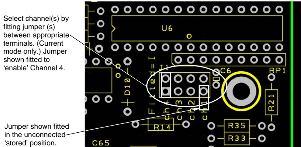
Figure 4-3. Location of Jumpers on Circuit Board
