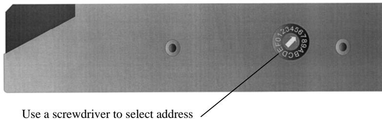
*Figure 4-4. Address Selection Switch*
