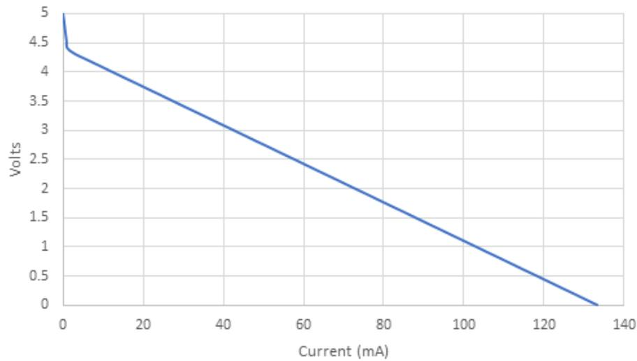
d) Output voltage versus current output
