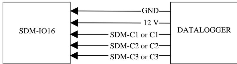
a) Connection with Datalogger Supply
