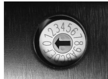
Figure 5. Address Selection Switch
