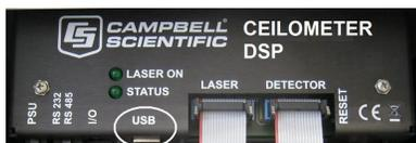
2. Use a terminal emulation program to set baud-rate settings to 115200 baud, 8N1
