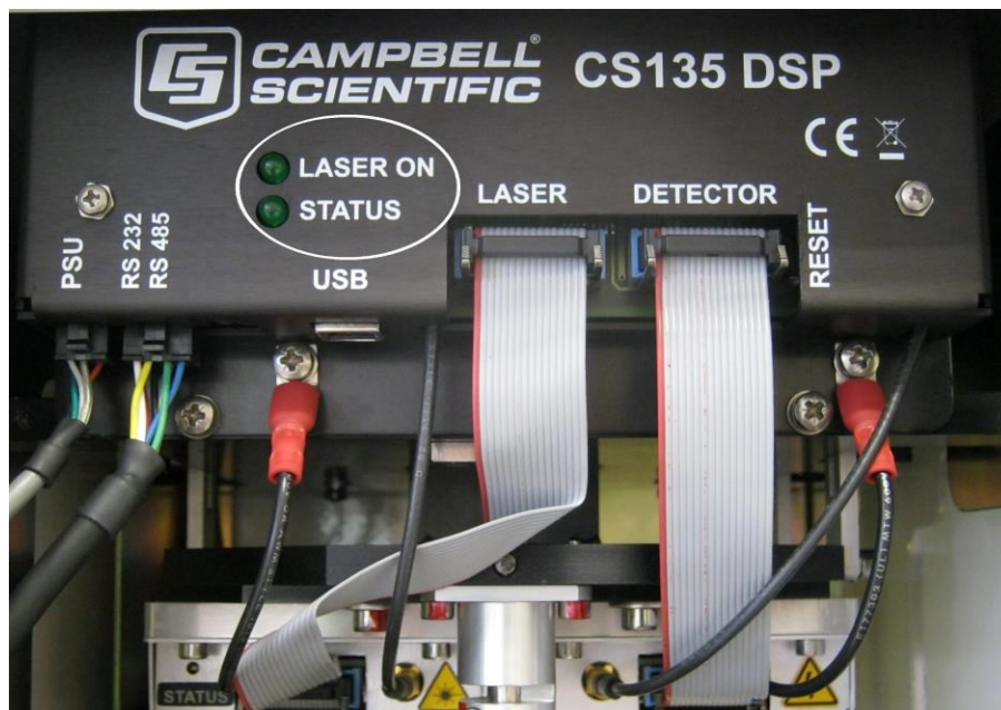
FIGURE 7-3. Diagnostic LED indicators
