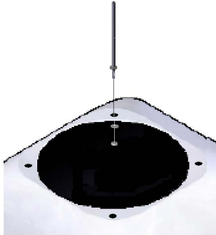
FIGURE 4-11. Attaching bird spikes to the SkyVUE PRO cowl
