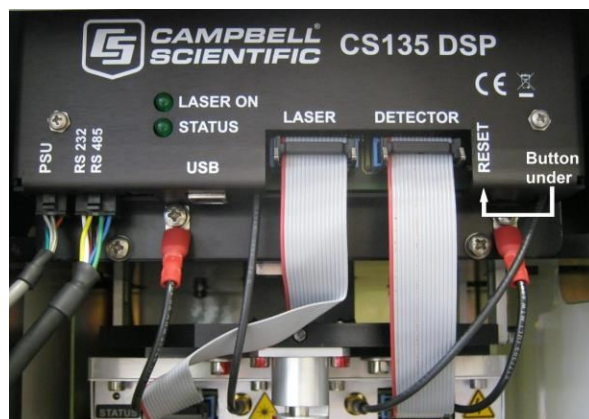
FIGURE 5-1. Restoring factory defaults
