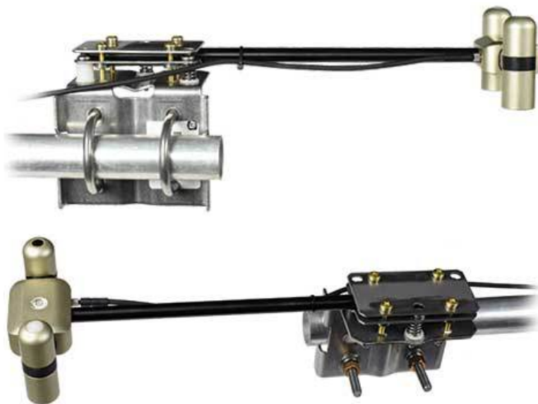
FIGURE 7-3. Two views of the SN500SS mounted to a horizontal crossarm
