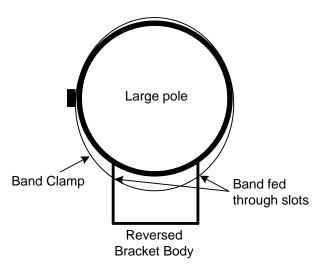
Figure 4. How to attach the multi-fit bracket to larger poles using a band clamp
