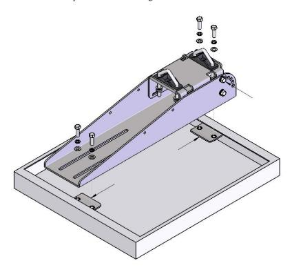
Figure 3a. Assembly drawing for fitting the multi-mount bracket to a larger panel
