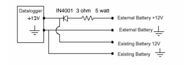
Figure 6. Connecting to External Power Supply
