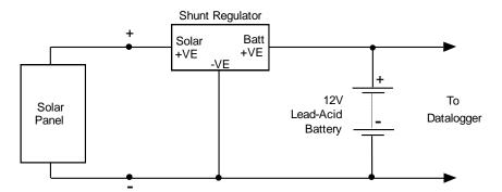
Figure 5. Connection of Shunt Regulator for SP10R Panels
