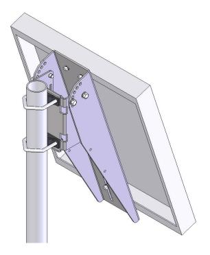
Figure 3b. Solar panel mounted on pole using the multi-mount bracket
